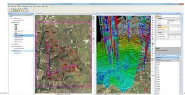
cross section, and 3D view of a geomodel which enables you to work in 2D or 3D views simultaneously. Using the Geo Surface Model tool, efficiently handle and update linked and complex geometries on all the views of GVERSE Geomodeling.
